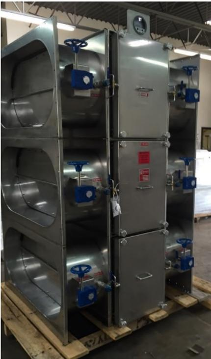
*CTC Model B1-212-3x2-RCD22x48 (above), with round or oval dampers which are difficult to insulate and ship without risk of damage. Best to insulate in the field (after making duct connections) using a soft-wrap, insulation, as pictured below on a B2-series housing w/dampers.*
