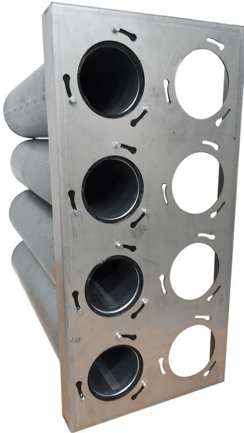
**HEGA (High-Efficiency Gas-Phase Air) Canister Filter Housings** utilize a heavy-duty 12"x24" holding frame to hold the canisters and allow for high-airflow with very low pressure drop. The canisters are gasketed on the side-wall and then slid into the 2" deep filter channel to provide a bypass-free installation in the side-access housing. Canisters are perforated on both the inside and outside and can accept any type of granular or pelletized gas-phase media.
