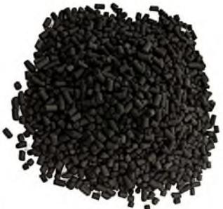
**HEGA (High-Efficiency Gas-Phase Air) Medias** are various granular and pelletized medias that can put into perforated trays or canisters. Media selected is based on the gaseous-contaminants that are to be addressed. Sometimes medias must be put into consecutive beds to address gaseous-compounds or for high concentrations of certain gases or compounds.
